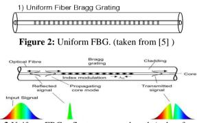
Figure 3: Uniform FBG reflects one wavelength.( taken from [5] )
