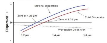
Figure 1: Zero total dispersion at 1.31 micro meter in step index SM fiber.
